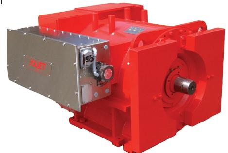
The Joliet Horizontal AC Drilling Motor delivers a continuous 1500 HP rating for mud pump and rotary table applications and boasts an impressive intermttent rating of 2250 HP for drawworks duty. The continuous rating is at 600/690 VAC, 1350 Amperes, 45.6 Hertz, 900/1800 RPM.
